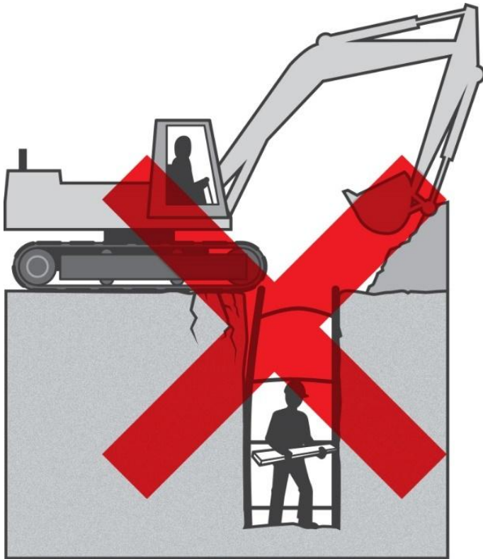
Figure 10 Large earthmoving machinery should not be operated close to an excavation
