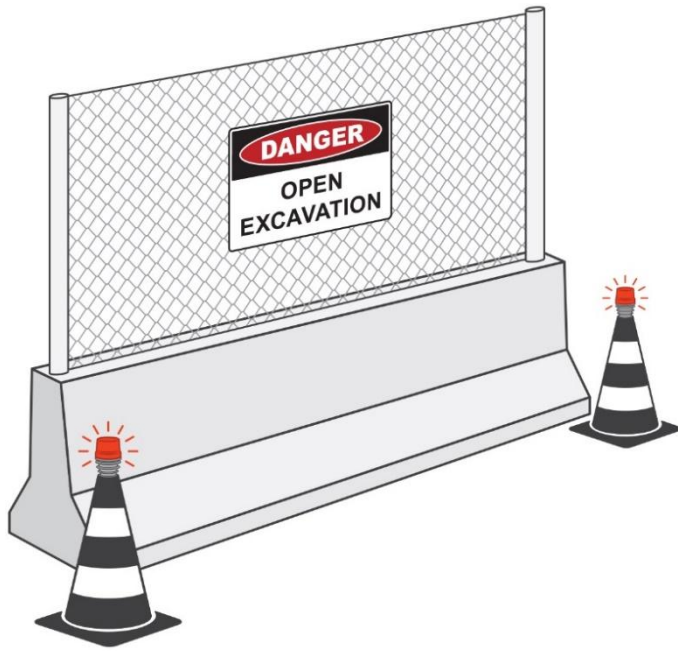
Figure 8 Barrier fencing and signage
