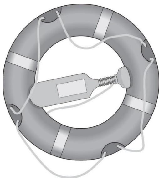
Figure 4 Life buoy with rope storage cannister
